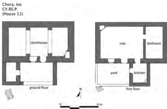
Fig. 6.80 Plan of an extended L-shaped type of the broad-fronted house (No. 11), Chora, Ios
