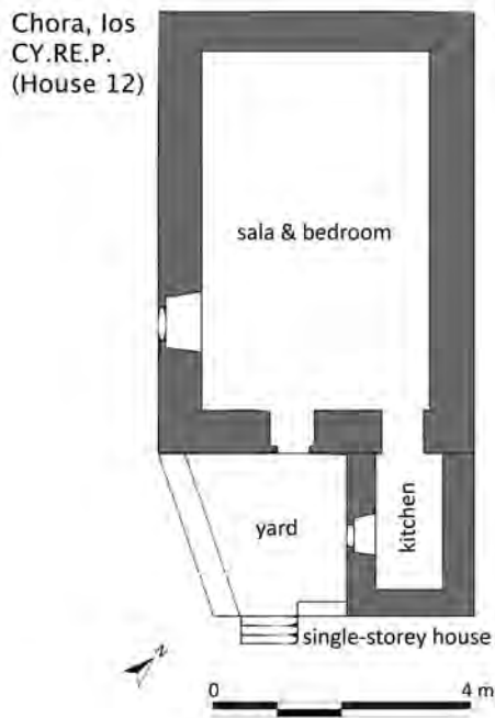
Fig. 6.82 Plan of an L-shaped version of the single-storey single-roomed house (No. 12), Chora, Ios
